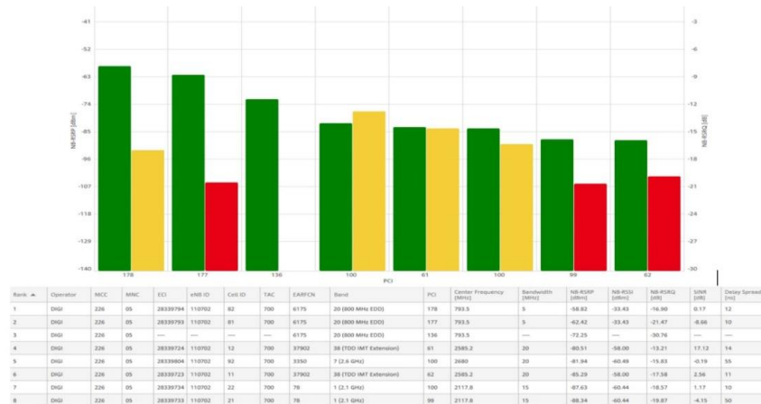
Figure 7.29. NB-RSRP, NB-RSRQ and other Digi Mobil downstream connection data at the radio monitoring point, obtained with the Nestor monitoring platform.
