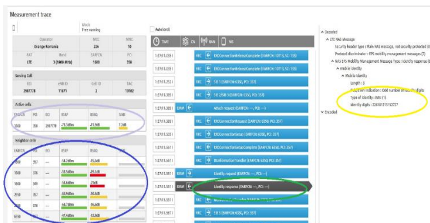
Figure 4.4. Successful completion of authentication and IMSI transmission.
